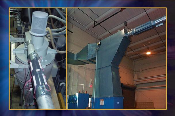
Liminate troublesome, static-induced clogs from your trim and waste handling system with our BarStat Ionicflow System. An integral part of your automated PAC system, it neutralizes charged paper, plastic, textiles and other chopped or granulated materials to keep them
