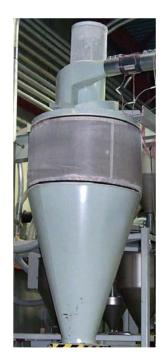
As paper, plastic, textiles and other trim and waste materials race through the trim system, they often develop a static charge as they approach the air separator. If the voltage is high enough, it causes the waste to cling to the air separator and to each other and could even become a hazard to plant personnel and equipment.
